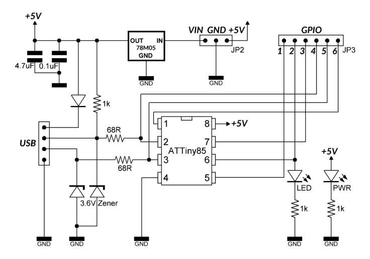
The schematic diagram shows the simplicity of the Digispark circuit. The circuit consists of an ATTiny85 chip, voltage regulator, diodes, few resistors, capacitors and LEDs.
