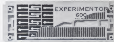
Both models feature 94 five-point terminals (vertical lines) and two 48-point bus strips (one strip shown).
