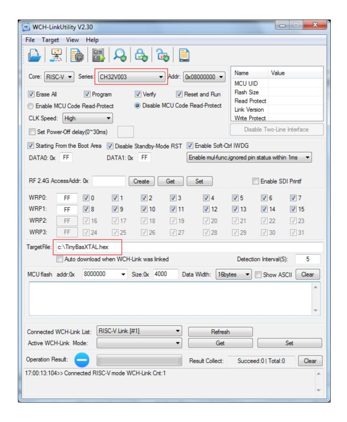
There are 2 versions of HEX files in the Bin directory. The user must decide which version to use. If the crystal is planned to be mounted on the board, select the program "...XTAL...". If the crystal will not be used, download and load the version "...RC..." into memory of CH32V003.
