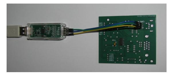
If necessary, the processor content can be overwritten with a new version in the future. The keyboard must not be connected to connector J2 during programming!
