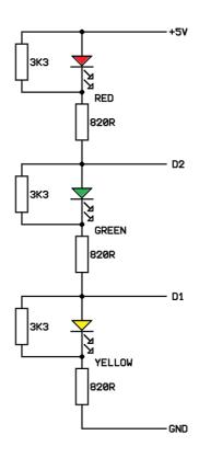
The green LED, even though it is located at the bottom of the traffic light, must be electrically connected between the red and yellow.
